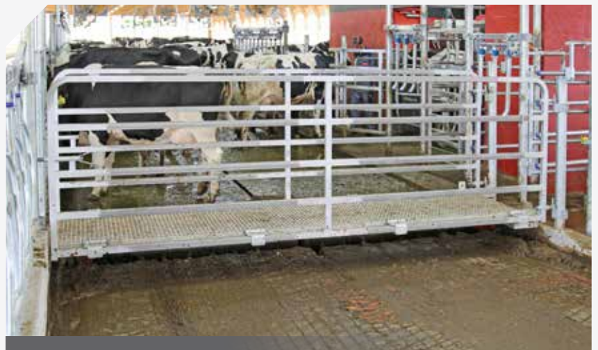
Clean Access Man Walks - Hinging gate with folding deck allows the manwalk to swing aside for scraping and equipment access
