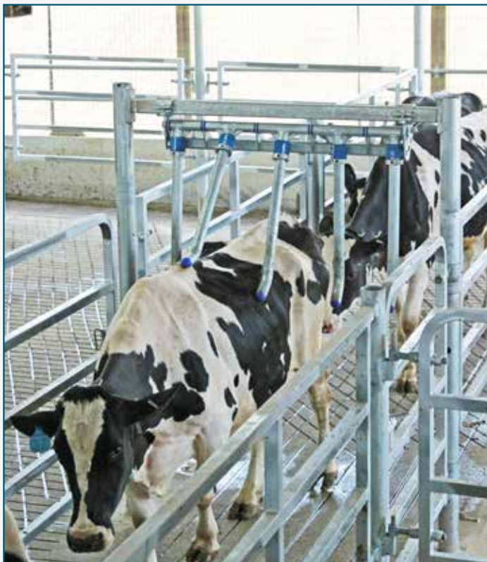
Stationary One-Way Flow Control Gate
