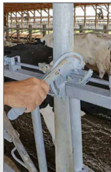
Control Latch is clamp-on for convenient positioning
